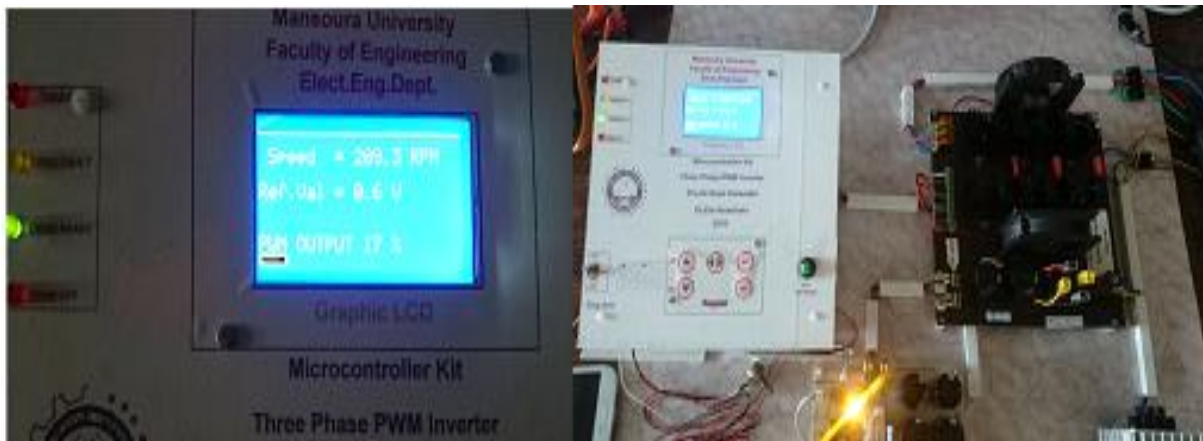
Figs. 17 Power and Control Circuits of ACIM Drive Laboratory Boards
